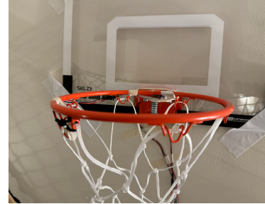
Figure 6: Line Break Sensor Mounted on Hoop
